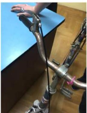
EN After positing the cable brake into the hand brake, reposition the brake lever in its standard position.
