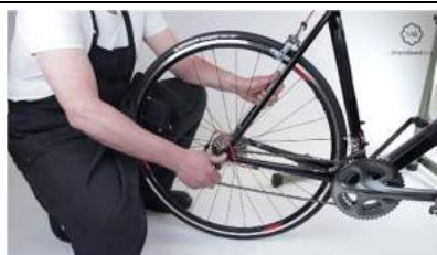
EN Bolt with fingers both record nuts and check the result.
