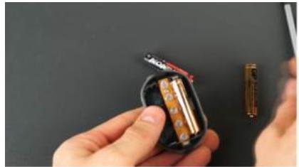
EN Insert the new batteries, respecting the + / - symbols.
