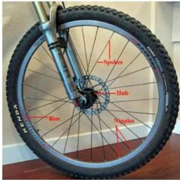
**EN** The wheel is one of the main components of the bike, a circular component that is intended to rotate and drive the bike forward. There may appear problems if the wheel wobbles side to side, or isn't perfect during braking. The wheel can clip off the frame and cause problems or accidents.
