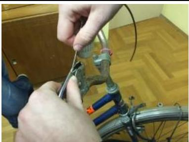
EN After checking if the brake works properly, assemble the brake cable. Do it manually, using a screwdriver.
