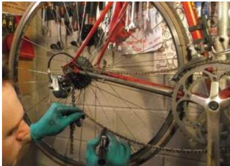
**EN** Approach the two final links and graft them in the chain breaker tool. Insert the lock latch with your hand and then push it inside with the puncheon of the chain breaker. Shimano's pawl has a first flared part which allows you to centre the holes of the plates and to expand them up to create the interference. Lubricate the chain.
