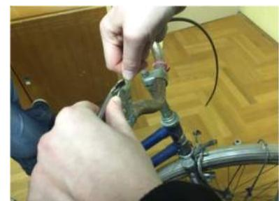
EN The brake cable has to be inserted in appropriate bearings on the hand brake. Tighten it.
