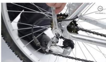
EN Tighten the nuts with spanners and check the result.
