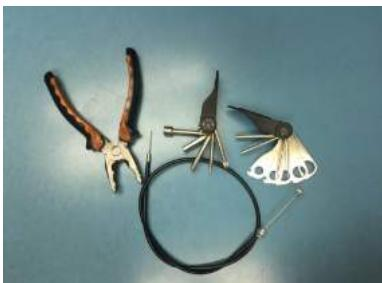
EN To replace the brake cable, you need: a brake cable, side cutting pliers, screwdriver set (Imbus set).
