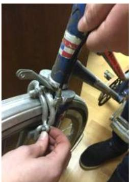
EN Tighten the cable using side cutting pliers and screwdriver by adjusting screw.
