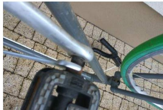
**EN** Tighten the screw with a screwdriver. Turn left pedal to left and the right pedal to right.
