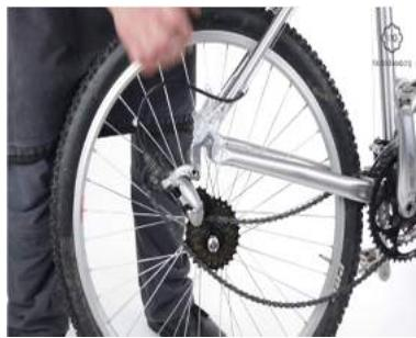
EN Place the wheel between the frame bars using spanners for adjusting.
