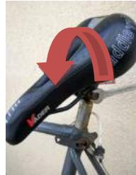
**EN** Loosen the bolt until you can move the seat.
