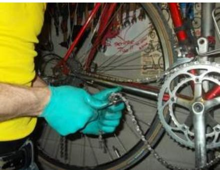
**EN** Controll the size of the new chain. Mark the size of the chain making a point on the terminal pin. Insert the chain, making it pass on the rocket and both derailleurs. Remove the links in excess expelling the pivot that you have marked. Take the lock pawl/latch which is supplied with the chain.
