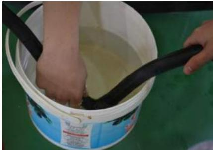
EN Remove the bike wheel and take out the inner rubber tube. If you don't see any obvious punctures or blowouts, inflate the tube so you can check for escaping air. To find very small leaks, pass the tube close to your eye to feel for air or submerge it in water and look for bubbles.
