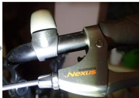
**EN** Turn the adjusting screw of the brake handle in as much as possible (don't break it).
